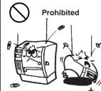
■ Do not insert or drop metal, flammable or other foreign objects into the machines through the ventilation slits, as this may cause **fire** or **electric shock**.
